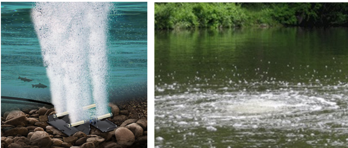
Figure 48: Diffused aeration system shown from the bottom of a pond/lake (left) and surface (right); taken from ProPond and Lakes (2021).
